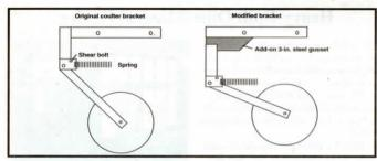
Barry Boggle, Hamilton, Ontario: "The shear bolt on the coulter on our Deere 2700 plow would shear often when we set the coulter at a lower angle to cut cornstalks better. We solved the problem by cutting the coulter shank off the main frame and inserting a 1 by 6-in, steel gusset that lowered the coulter by 3 in. This lessened the angle, shortening travel of the spring. It works so well Deere personnel even came out from the factory to look at and measure our modification.
