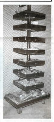
plate to make a larger bottom tray that bolts to the axle hub's five studs so that the axle housing and seven travs turn freely. I put a bracket at the top that screws to the wall to hold the entire unit stable. If I need to roll the trays to a different place in my shop I just push up on the bracket to release it.
