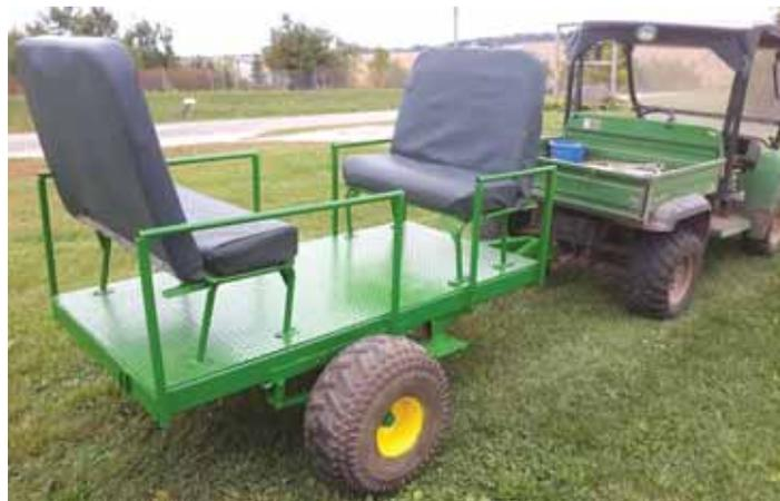
Dykstra fabricated the steel frame and platform and mounted it over an axle and leaf springs from an old boat trailer. The wheels were salvaged from a junked 4-wheeler, and the seats came out of an old school bus.
