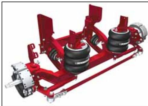
Improved features include shorter aluminum beams to reduce packing space, a compliant tie rod to resist permanent deformation and enhance adjustability, along with an optimized package design with shorter trailing arms and side rails.
