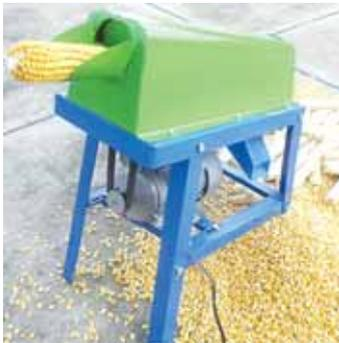
Operating at a speed of 2,800 rotations per minute, it takes about 3 to 5 seconds to thresh each ear of corn.
