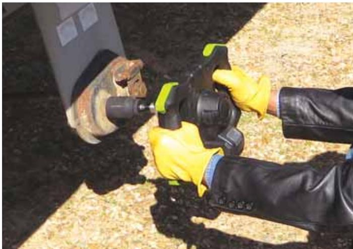
Torque elimination device makes opening hopper doors on grain trailers easier.
