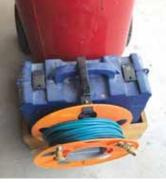
Strayer used some extra air chucks for an extension to make draining the tank easier. He also added a tool box and cord reel for hose storage.
