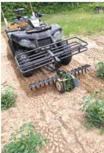
**"I added mounts for a set of wheels from an old rototiller to the bar, giving the tines about a 1 1/2-in. depth. I also added galvanized aluminum shields inside the wheels to keep from running over plants," says Sieting.**
