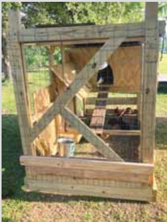
**Reaux designed the portable building to be easy to maintain. It's tall enough to walk inside, but he has outside access to the roosting box to clean it out into a wheelbarrow.**
