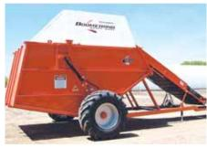
The Boomerang 30 holds roughly 2 tons of material. Rather than the floor dropping to the ground for unloading, only the rear gate opens and closes with hydraulics.
