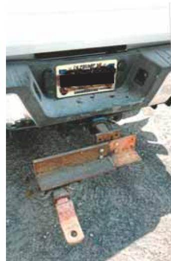
**Barley designed a hitch that goes in the receiver to move it about 16 in. to the left. It really helps to keep the outside wheel on the road more.”**
