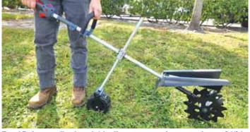
TrenchBadger can slice through 1-in. diameter roots and cut a trench up to  $5\,1/2$  in. wide and 12 in. deep when using both blades.
