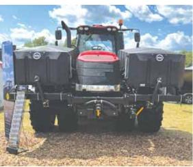
Designed for Deere 8000R tractors, tanks can be installed on some Case IH tractors as well.
