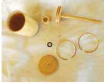
**Tiny pistons, rings, sleeves, and other engine parts are all made of wood.**
