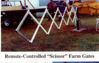
You'll like this new electrically-operated scissors farm gate featuring remote control for easy operation from an ATV, tractor, or pickup.
