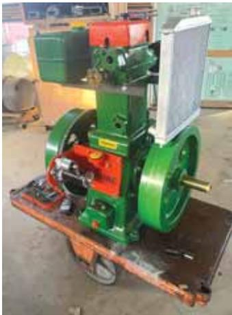
**Running at a top speed of 1,000 rpm's, these engines can run 8 hrs. at 35 percent load and use just 5 quarts of fuel.**
