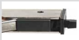
Ronald Hurst, Knoxville, Tenn.: "This is a handy, fairly inexpensive tool that turns a round hole (3/8 in.) in sheet metal into a rectangular hole, any size. I use my nibbler mostly for squaring holes in electrical/electronics projects (holes for things like digital displays, fuse holders, snap-in rocker switches, etc.).
