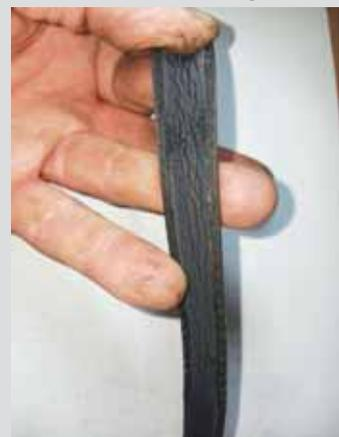
Dale McLaen, Rutland, N.D.: "Repeated plug-ups in the fuel filter between the tank and carb caused me to follow the fuel.
