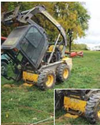
Cut out door makes cleaning out the chassis easy.
