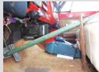
Grady Hurst, Knoxville, Tenn.: "For lack of a better name, this is a 'Pedal Presser Downer' tool. You press down the gas or brake pedal of a car or truck and put this tool in place to hold the pedal down. This idea came from an auto mechanic whom
