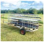
Arcement had the frames, and putting them on a boat trailer made the concept more user-friendly. The trailer, which once carried a small aluminum boat, was wide enough to mount one tote frame at the rear over the 12-in. wheels.
