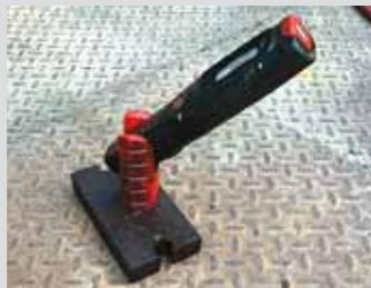
**John Rochester, Charlotte, N.C.:** "To make it easier to work hands-free in tight spaces, I attach a heavy chunk of metal to the magnet base of my rechargeable wireless work light. Holds it solidly in place.
