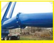
I bought this Brandt auger from an insurance company for \$2,750. It had been damaged and had a big kink in it so it couldn't be used. To work on it, I put the auger wheels in a ditch so the auger tube was at waist level. Then we straightened out the tube and repaired the bent auger flighting. Once we finished, we had a nearly new auger worth \$50,000. (Roger Gutschmidt, Gackle, N.D.)
