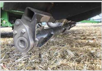
Devastator uses flat steel roller bars that knock over stalks and crimp them as the combine moves through the field.
