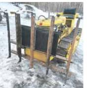
Vertical bars are pointed to pick up brush tight to the ground. Draw pins make changing back to the dozer blade quick and easy.
