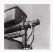
Extender mounts between motor and auger tube, protecting motor from direct contact with fertilizers.
