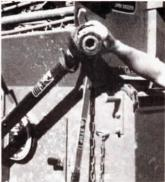
New Snap-On coupler is easily hooked up with one hand.
