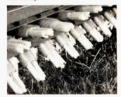
The optional conditioner has nylon brushes which scratch wax covering off crop to speed drying.
