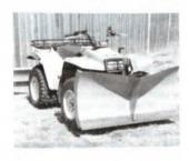
in FARM SHOW. We now have mounting brackets so it can fit onto the Deere Gator utility vehicle. The split blade rolls snow left or right with less side draft than conventional plows. A 12-volt electric linear actuator eliminates hydraulic hose problems. (Trail-Buster Dozer, Inc., 272 Main, Grainfield, Kan. 67737)
