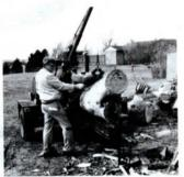
and lower the boom, rotate it, and operate the winch. If I'm not using the boom or winch I can close the flow divider valve and divert all of the oil to the log splitter so it works faster. The cutting table on the buzz saw is hinged so that I can flip it up out of the way for over-the-road transport."
