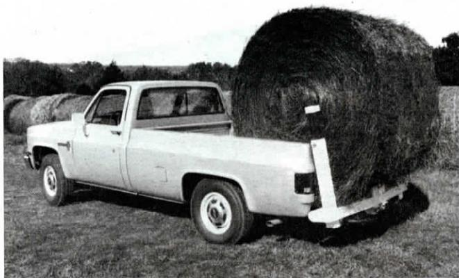
Bumper's hydraulically-powered arms swing out to grasp bale.
