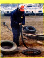
Conventional 15 in. car tire, cut into 2½ in. wide strips, produces continuous fencing strip 40 to 50 ft. long. Owners of the new fence-making machine say they get all the used tires they want, free of charge.
