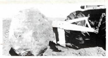
Note small prongs on the lower rear side of the shanks which make it easy to push large rocks out of their resting place after they have been loosened.
