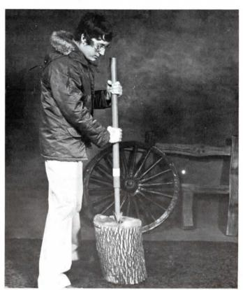
Slide-hammer action drives wedge point through the log with a minimum of effort.
