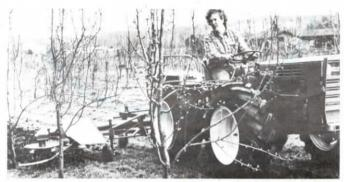
When the ultra-sensitive sensor — the brain of the Cultimatic — touches the tree trunk, the cultivating arm draws back about 14 in. to clear the obstacle. Once cleared, the twin rotors return to their original position.
