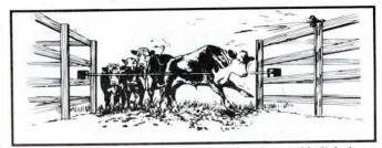
When livestock enter fence opening, they break invisible light beam which activates flashing light and horn.
