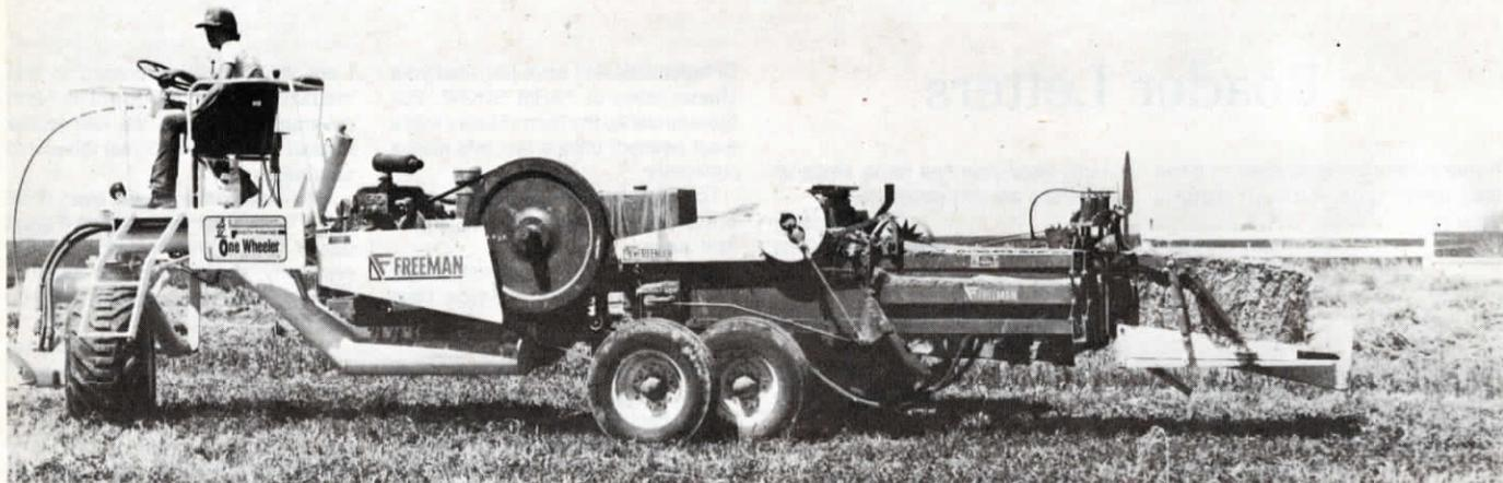
Adapter plate allows "One Wheeler" self-propelling system to be transferred from baler to swather to other pull type equipment. It features fully hydrostatic drive and excellent maneuverability.
