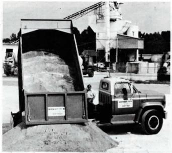
Bed rotates 180°, allowing the box to be raised and dumped at any angle, whether completely sideways, straight back or anywhere in between on the 180° axis. Driver can rotate and dump box while truck is moving.
