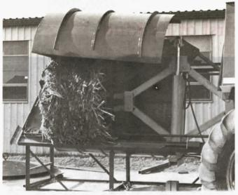
In above photo, toggle arms of the compactor will eventually become horizontal as the machine fully compacts a 6 ft. long bale (6 ft. dia.) to 2 ft. Photo below shows the bale after being compacted and the arm withdrawn. Steel bands secure the compacted bales.
