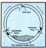
Six of the three "input" openings built into the outer circumference of each ring can be regulated by inserting plastic plugs. As disks rotate, dry material is picked up by the openings and channeled via rectangular-shaped grooves to the "output" openings. Individual disks are ganged to form a drum, with solid disks at each end to seal the drum.
