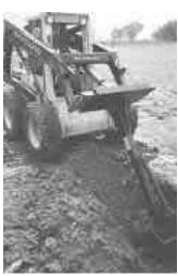
The Skid-Digger bolts in place of the bucket. The angle of the backhoe is set with a pin.
