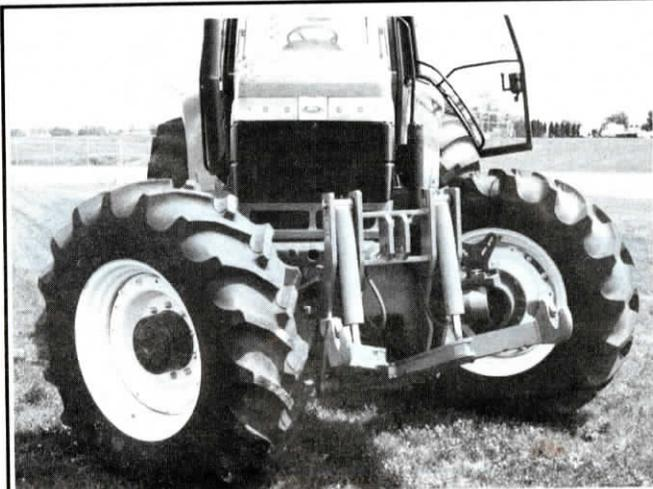
LaForge Systems, Concord, Calif., specially designed this front-mount 12,000-lb. capacity 3-pt. hitch for the new "SuperSteer" axle on Ford's Genesis tractor. The axle-mounted hitch allows implements to take full advantage of
