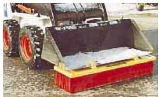
Broom head is equipped with 10 strips of 10-in. long poly bristles. Strips slide into tracks built into broom head.
