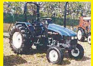
The new 35 Series tractors range from 56 to 86 pto hp. Like the larger 60 Series, the tractors have sloped hoods for better visibility. They come with a choice of three different transmissions, each with forward/reverse shuttle. New Holland says Series 35 cabs are bigger and quieter than most other models on the market, and more convenient to use with tilt steering and two doors.
