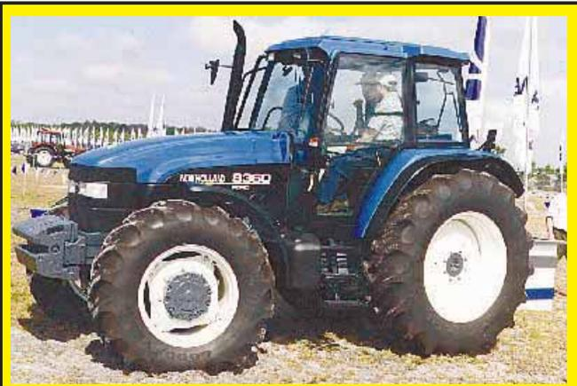
The 115 hp. 8360 is one of four models in New Holland's new "Gemini" 60 Series that ranges from 90 to 130 hp. All four tractors feature the New Holland-built Genesis 7.5 liter, 6-cyl. diesel engine. Available in 2 or 4-WD with a choice of three different transmissions. Cabs on the new tractors are wider than competing tractors and the sloped front hood and narrow chassis provide better visibility, according to the company.
