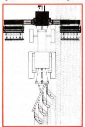
You can plow, till and plant in one operation. Front-mounted seeder, on right, seeds previous round's plowing strip.
