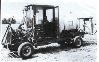
Self-Propelled Sprayer Features Stand-Up Cab
