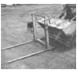
quickly between the bucket, for loading silage out of my bunk, to the spears for handling big bales."
