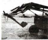
I designed and patented this ditch hoe for front-end loaders. It digs a ditch 6 to 12 in. wide to a depth of 54 in. What makes the digger unique is the way it dumps dirt to the side of the ditch. The digger arm mounts on a metal tube that's rotated by a hydraulic cylinder. The bucket makes a 180° arc as it digs a bucket of dirt, then moves to the side to dump when the cylinder reverses rotation of the tube. Bucket then returns to digging position for another pass.
