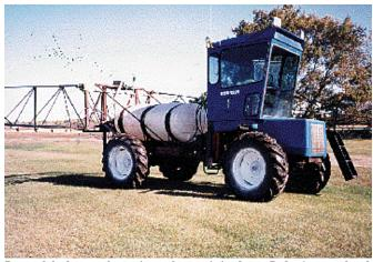
Roy used the frame, axles, engine, and transmission from a Dodge 1-ton truck, cab from a New Holland combine, and flotation tires from a Massey Ferguson combine.
