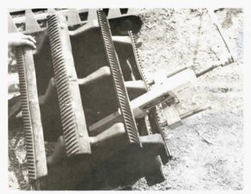
It only takes a few seconds to insert the "jig" and turn its straightening screw to iron out bent rasp bars.
