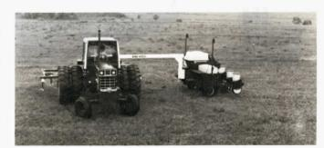
Hydraulic hoses from planter are threaded inside the hollow Bink Hitch.
