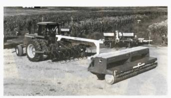
Bink Hitch allows three 8 ft. drills to be hooked side by side behind a digger, rotary, field cultivator or other tillage tool.
