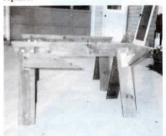
Earl Rahn, Beaver Dam, Wis.: "I've found these fold-out extension arms, mounted on one of my wood sawhorses, to be a big help, especially when sawing 4 by 8-ft. sheets of plywood. There's a fold-out arm at each end of the sawhorse, mounted on a heavy hinge. The upper end of the arm is cut at an angle. When needed, you just fold them out and they act like a third sawhorse. When you're done, they fold flat, out of the way, so you can still stack the horses normally for storage.'
