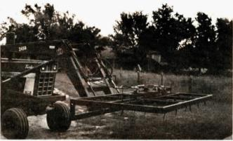
I can pick up 15 bales at a time with this bale "grab" I built for taking bales out of a New Holland bale stack. I also use it to add three layers of bales to stacks when I'm haying. Carrying capacity could easily be increased to 18 bales for New Holland's larger self-
