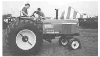
Norm Craigie's Deere 4320 runs on a blend of 20 percent soy oil. It has placed high in tractor pulls two years in a row.
