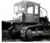
We built a cab for our D6 Caterpillar from scratch to our own specs. The main frame
