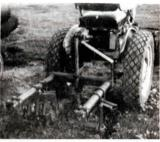
welded two 1-ft. long steel bars onto the truck axle at the same angle. On the left side, I welded on an upright steel bar (about 1 ft. long) so that the tractor lift could be hooked up to it. The bars on the truck axle have two turnbuckles that hook up to each Ford drawbar lift arm. To make the top link I removed the tractor battery and seat and bolted a steel plate to the tractor, then replaced the seat and battery.
