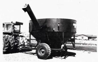
No supports are needed inside the round cart. Wet grain gravity feeds out bottom without bridging.
