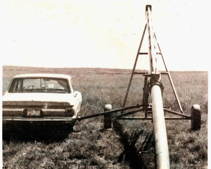
Frost uses a 1965 Plymouth to power grain augers. Shifting gears lets him change auger speeds.
