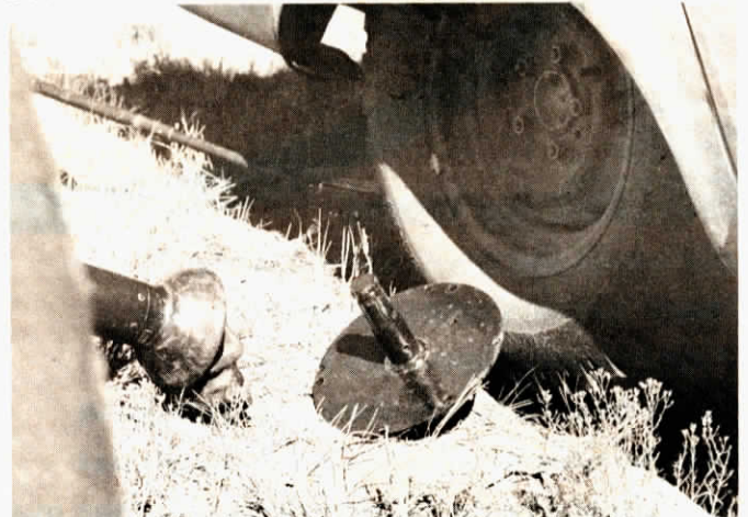
Pto adaptor plate simply bolts to car wheel with three bolts.
