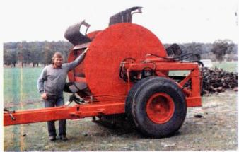
Curved steel tines sift through soil to pick both roots and rocks.
