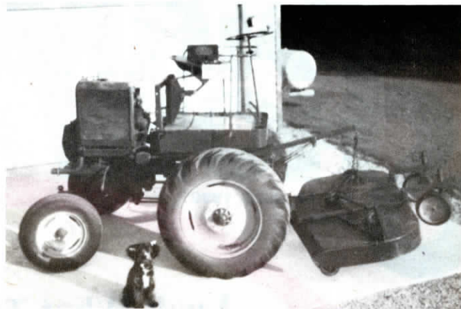
The deck is supported by a pair of cultivator gauge wheels and is raised and lowered by the same cylinder that formerly raised and lowered the header.
