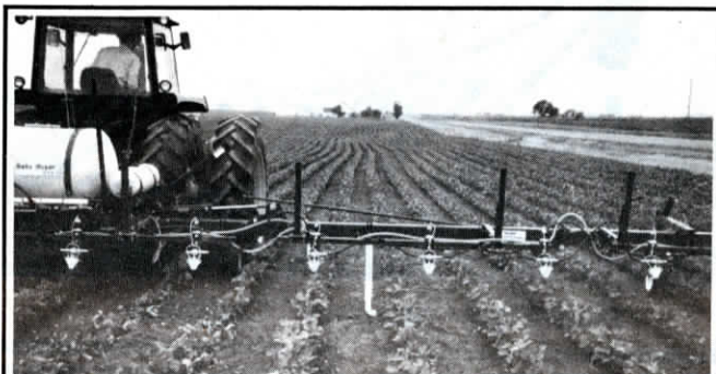
This early prototype was mounted on a crop sprayer. Unlike mechanical "wand-type" sensors, it reads off the crop without touching it.
