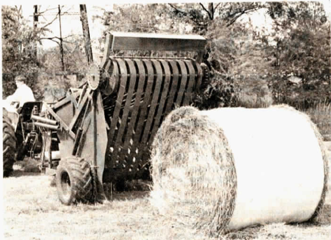
Hay pickup at rear of baler lifts to release the wrapped bale. Note interlocking ground-drive sprockets inside wheel and at either end of pickup reel.
