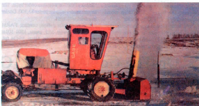
The blower is mounted on the original header lift but Buchholz added a tilt cylinder that lets him tilt the blower to either scrape or skid over the ground.
