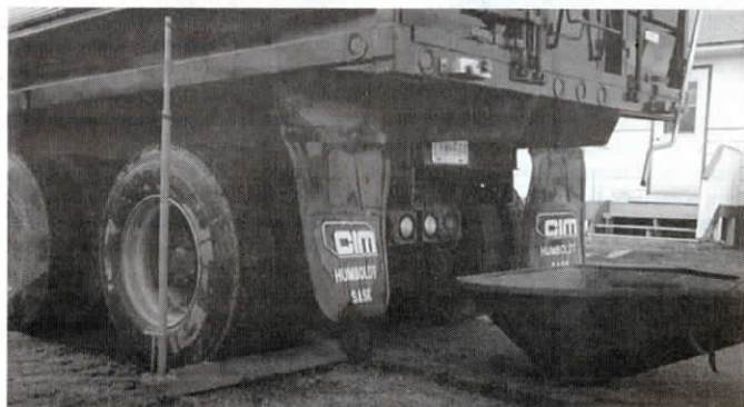
Truck tire bumps up against base unit, and pole keeps driver on line.
