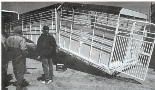
Back end of trailer lowers to the ground to load livestock. Racks come off to convert to flatbed.
